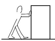
The person uses 30 N of force to push the box 10 m to the right. At the same time, the box experiences 5 N of friction.
