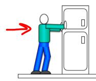
The person uses a force of 40 N to push the 100 kg fridge 4 meters to the right. Calculate the work done by the person.
