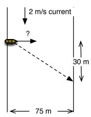
The motorboat is pointed straight across the river. The 2 m/s current carries the motorboat 30 m downstream by the time it gets across.
