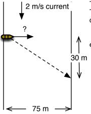
The motorboat is pointed straight across the river. The 2 m/s current carries the motorboat 30 m downstream by the time it gets across.
